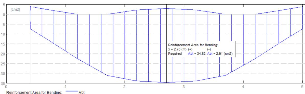
Fig. 2.1. Theoretical (required) areas of reinforcement in beam.
