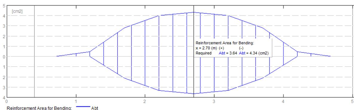
Fig. 4.1. Theoretical (required) areas of reinforcement in beam.
