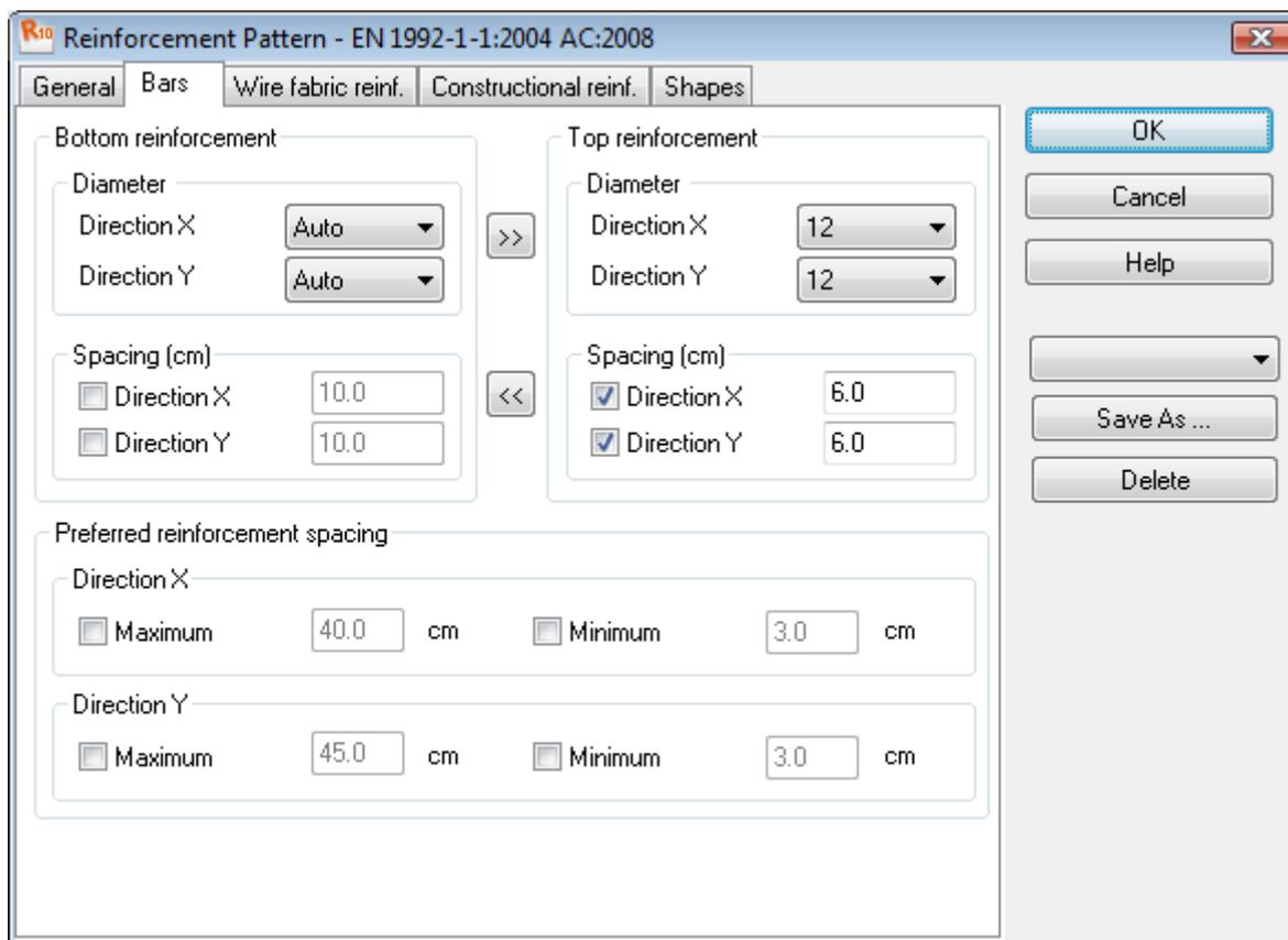
Fig. 4.4 Definition of spacing and diameters of reinforcement
