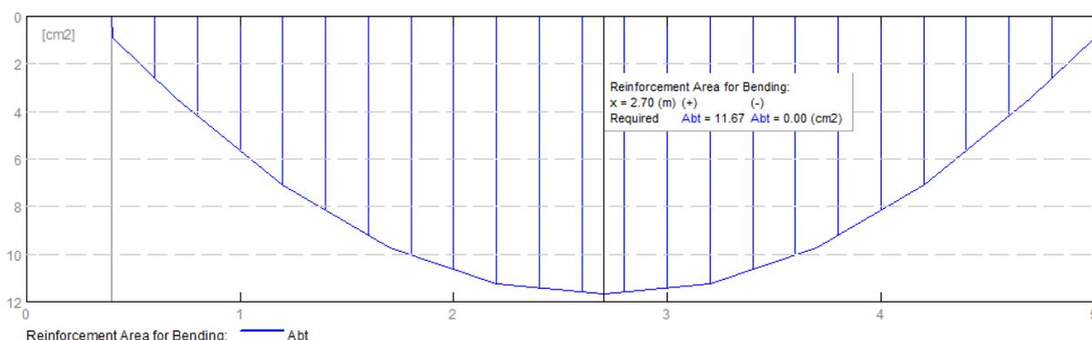
Fig. 3.1. Theoretical (required) areas of reinforcement in beam.
