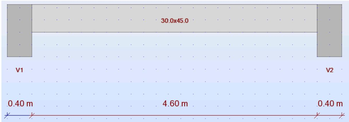
Fig. 1.1 Beam geometry
