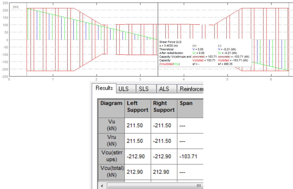
Fig. 5.3 Shear force distribution and shear capacity
