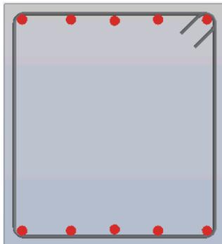
Fig. 1.9 Reinforcement assumed for the calculation (10  $\phi 20$ ).**RESULTS OF BUCKLING ANALYSIS - NOMINAL CURVATURE METHOD:**
