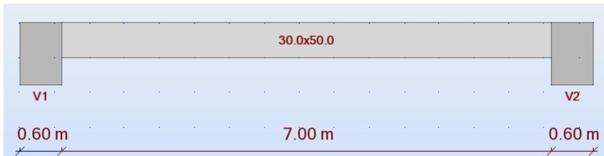
Fig. 6.1 Beam geometry
