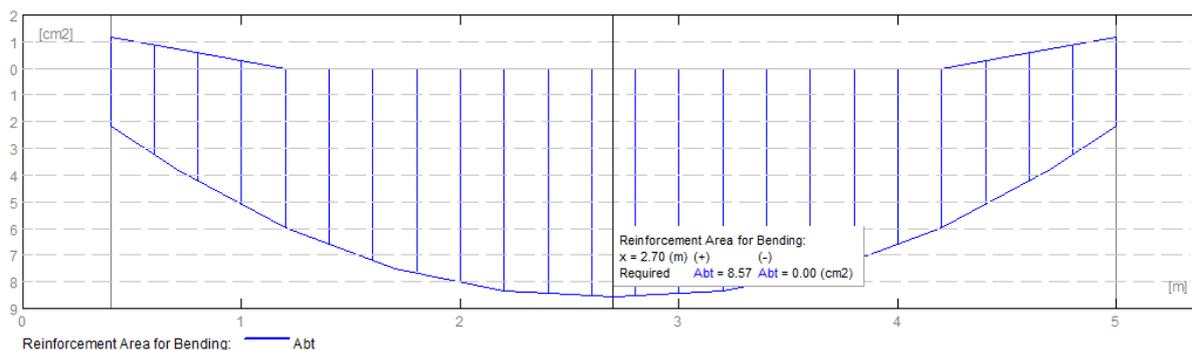
Fig. 1.5. Theoretical (required) areas of reinforcement in beam.
