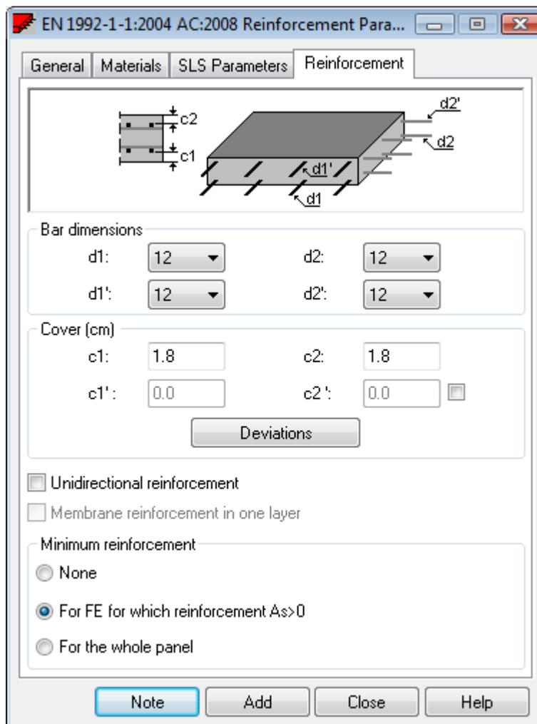
Fig. 4.3 Definition of covers of reinforcement
