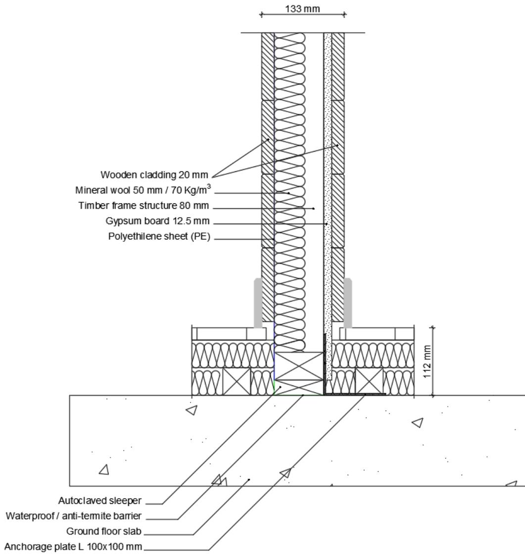
14 – TFS 105 – Floor panels composed of linear wood structure
