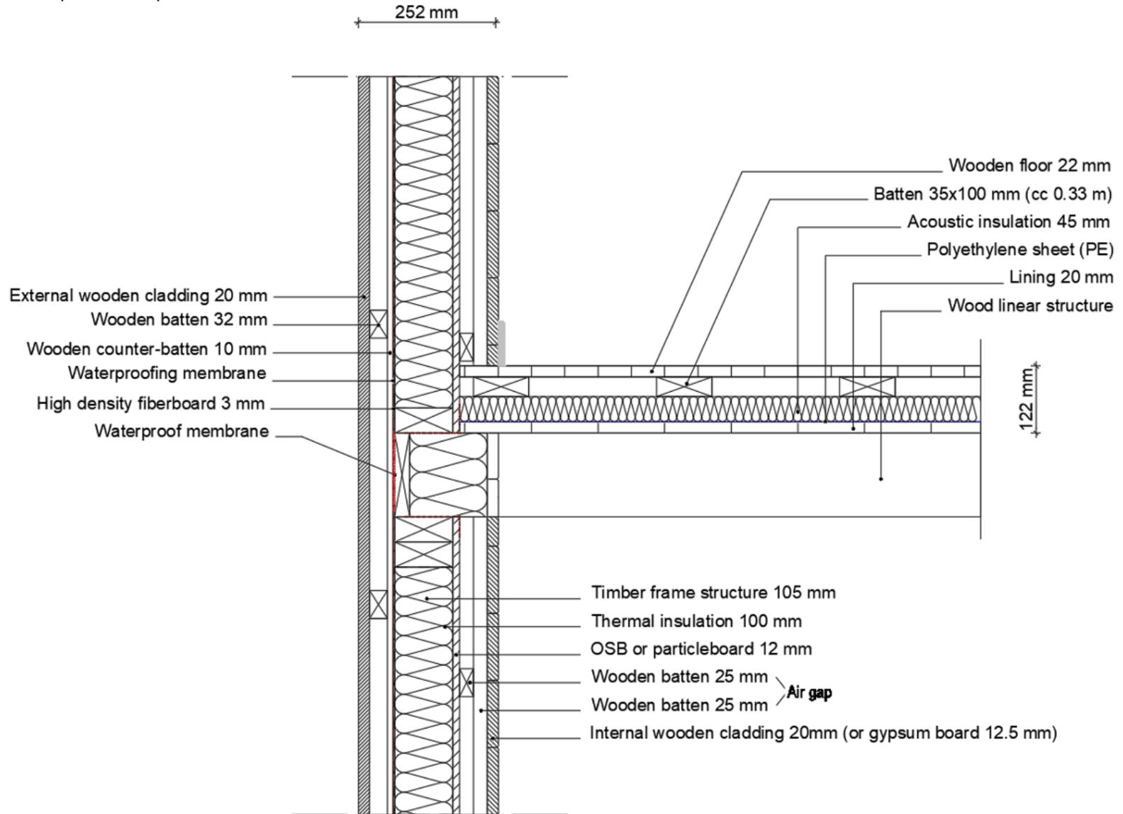
15 – TFS 145 – Floor panels composed of linear wood structure
