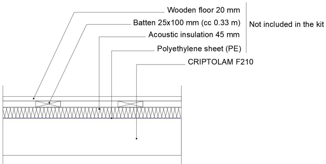
10 – Floor panels composed of linear wooden structural elements
